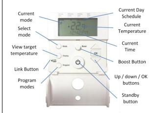
The Home Thermostat is used to control and schedule home heating. It Wirelessly links to Deta Connect Boiler Switch which turns on and off your boiler. If the Thermostat is also linked to the Deta Connect Link, you can also control and schedule your heating via the Deta Connect App.
