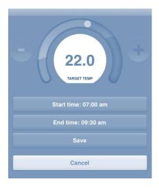
You can now choose a Setback Temperature. The purpose of the setback temperature is to allow your system to never get too cold; either frost wise when unoccupied, or uncomfortable when occupied (ie so you can come home early and it could still be 15C, even though the heating is 'off'). To set this temperature, select 'Setback Temp' at the top of your schedule
